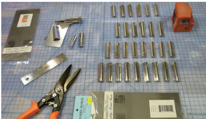
As you can see, a single sheet of #257 K&S aluminum is enough to make quite a few sets of aero shields.
