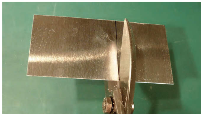
Measure and draw your lines. Cut the metal with sharp tin snips. Avoid stopping in mid cut to avoid any burrs or dimples in the metal.
