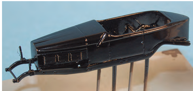
I like to use automotive lacquers but prefer spraying with my airbrush for better control, so I simply spray the rattle-can paint into a paper cup, let it sit for a couple of minutes, and then pour it into my airbrush bottle. Each progressive coat is thinned out with lacquer thinner until the final wet coats are not much more than colored thinner. The first color coat showed some rough spots, so it was sanded with #2400 grit cloth. Follow-on coats were sanded with #3200 and #4000 grit cloths between coats. Seats and interior panels were painted with Tamiya Flat red and semi-gloss clear to give them a realistic leather-like sheen.
