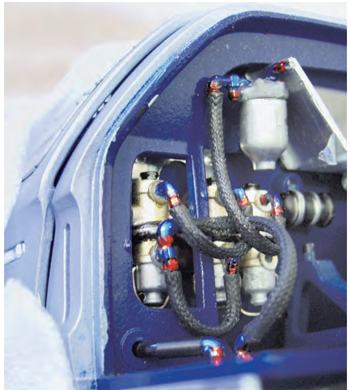
The fuel system also required some patience to get right. Shown above are the 1:1 fuel pumps mounted in a Cobra, and the 1:1 mounting on a restored GT 1046.
