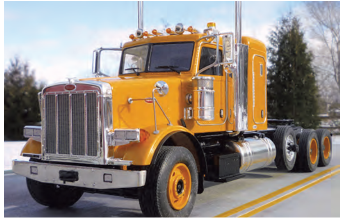
Aero shields look more streamlined than the stock shields. The roof mounted warning beacon mounts are also made from K&S aluminum bent to shape.
