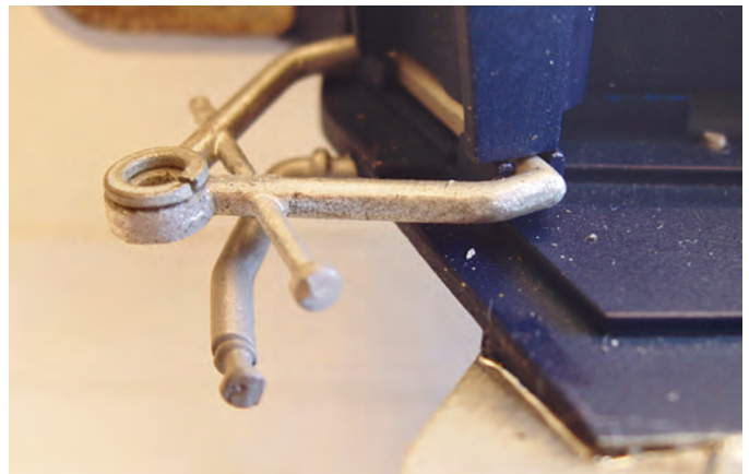
It was now necessary to raise the axle/upright assembly relative to the lower control arm. I found that a #6 washer placed on the lower control arm made a perfect seat for the axle unit and would raise it 1mm.
