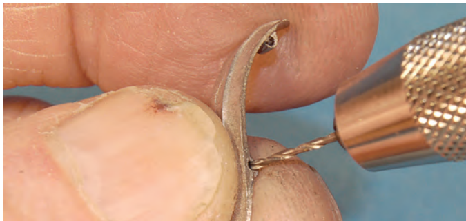
The pin vise was used again to make holes for the brass wire fender struts. Be careful not to drill all the way through the mounting nub.
