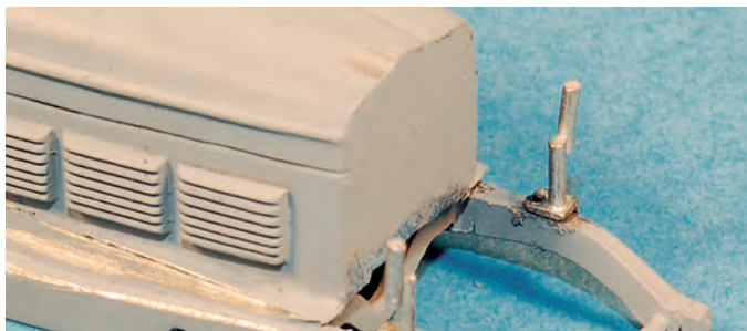
Headlamp supports were glued in place before the last primer coat. Note that the holes behind the bars line up with the holes drilled through the frame to accept the fender struts.
