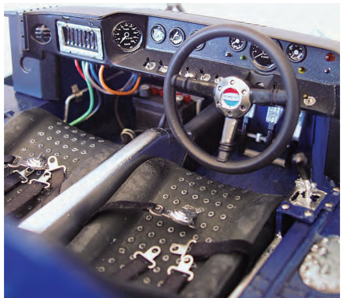
Above: The seats are Nato Black with German Gray dry-brushed wrinkles, and the seat vent rivets are touched with thinned acrylic silver. I shortened the metal steering shaft by .250" or the wheel would be in the drivers chest. Some cars used a speedometer to the left of the dash, and others put the battery master switch there—your choice.
