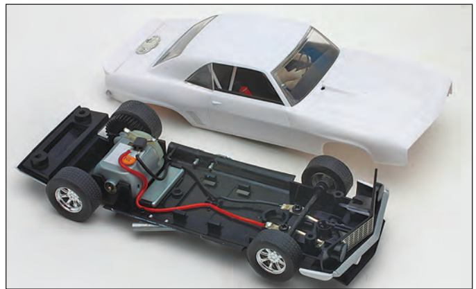
The stock sidewinder configuration is a perfect base for hop ups, tuning, and other mods. The chassis plate has one stock magnet (25mm x 8mm x 2mm), and two open magnet slots.
