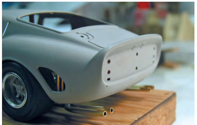
The nice thing about slot chassis is that they are usually built tough! However, when plastic is used for stuff that sticks out, it can be knocked off way too easily. For things like exhaust pipes it's best to use brass or steel. So a set of brass exhaust pipes shaped just like the kit parts were the originals stick out on the real 250 GTO.
